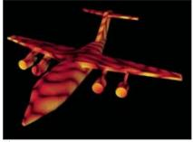
▲ Fig. 1 Surface current distribution on an aircraft.
